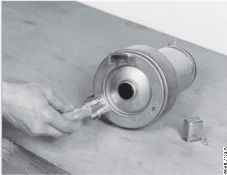
Figure 10: Pump feet removal
